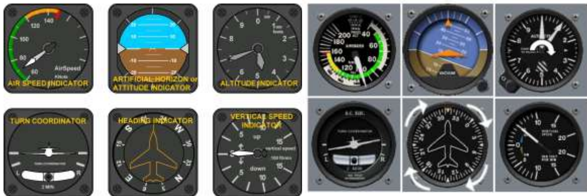
Figure 1: Experimental stimuli. Left panel shows the six main instruments (simulated) of Cessna cockpit used as stimuli in all experimental blocks except the “transfer” block. The instrument configuration indicates a “straight and level” situation. Right panel shows the instrument variation used in the transfer task. This configuration indicates a climbing left turn.
