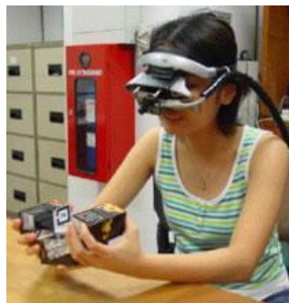
Figure 1: User wears a head mounted device (HMD) and views the 3D version of the story while exploring the contents of the story by unfolding the magic cube (Pan, Cheok, H. Yang, Zhu, & J. Shi, 2006).
