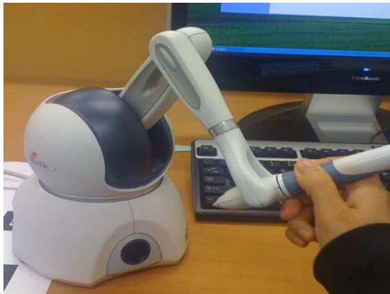
Figure 2: Phantom Omni robotic arm with ‘touch feedback’
