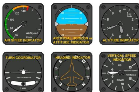
Figure 1. Six main instruments of the Cessna-based instrument panel used for stimuli in this study.
