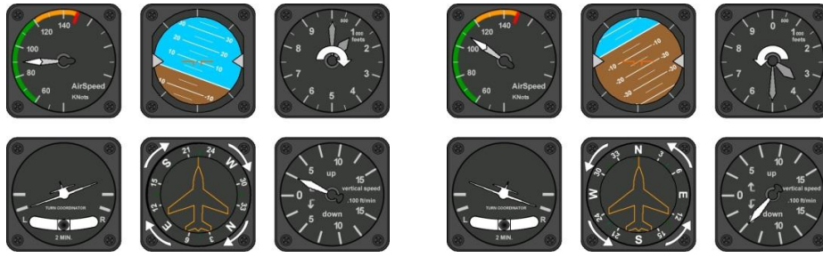
Figure 2. Left panel shows a climbing left turn whereas the right panel shows a descending right turn
